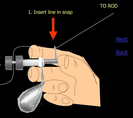
2. Push down as shown And insert line across clamp face
